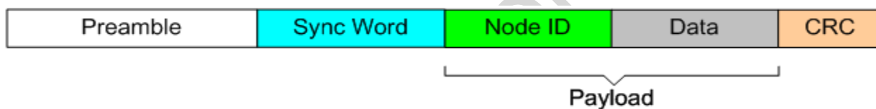
Figure 9. Packet Format for Packets with Fixed Length
